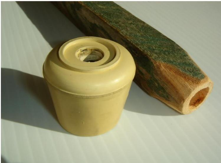
3. Insert the rubber leg tip to the end with the drilled hole.
