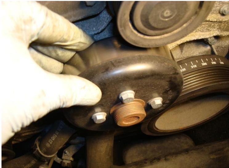
5) Next, pry the dust cover off the idler pulley with a small, flat blade screwdriver to expose the mounting bolt:
