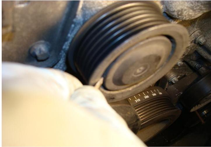
6) Using a T-50 Torx, remove the bolt – this bolt is long but only threaded on the end:
