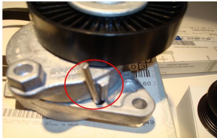
3) Using a 17mm wrench, push downward and counterclockwise to move the tensioner to its furthest position (that doesn't apply tension to the belt) in order to insert a pin into the tensioner. This is required to lock the mechanism so you can remove the belt as well as the old tensioner. Feel around with the pin for the hole because it's difficult to see. I used a large nail for a pin:
