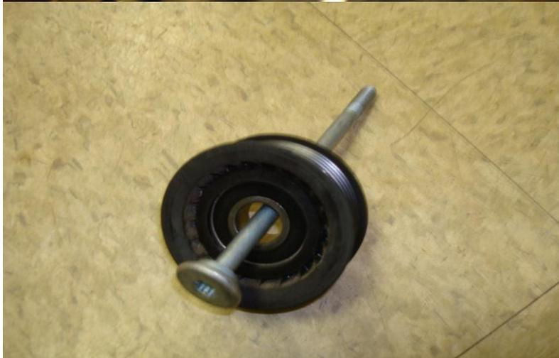
7) Clean the mounting area with a towel, and install the new idler pulley – there's no front or back but I like to have the part number visible. Torque to 20Nm (15 lbs ft).
