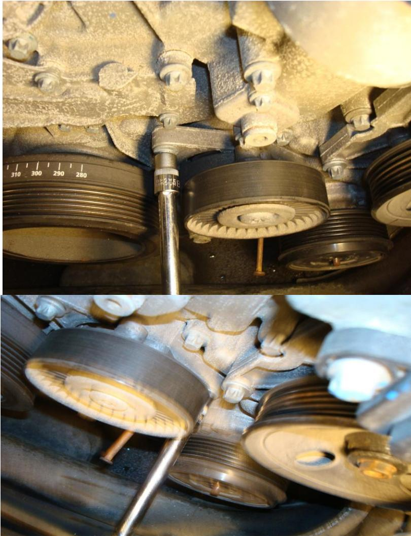
9) Once the old tensioner is removed, you may want to clean that area up and re-familiarize yourself where the mounting holes are. You may also want to clean up all the accessory pulleys (plain microfiber cloth or blow compressed air to remove any residual debris) as I found a good amount of sand/dirt in this area:
