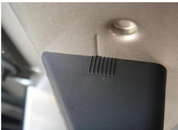
**NOTE: These adjustable wedges are actually boot lid guides and ensure a snug fit**
